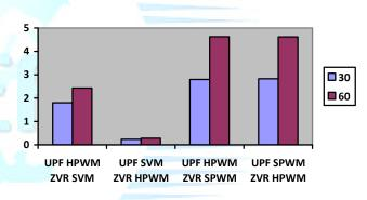
Fig 15. THD value of phase-A source current with two DSTATCOMs
