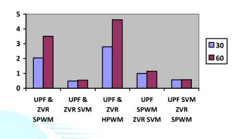
Fig 14. THD value of phase-A source current with two DSTATCOMs
