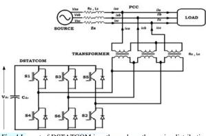
Fig. 4 Layout of DSTATCOM in a three-phase three-wire distribution system
