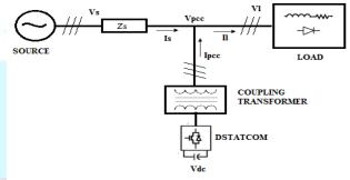
Fig. 1 Basic layout of DSTATCOM.
